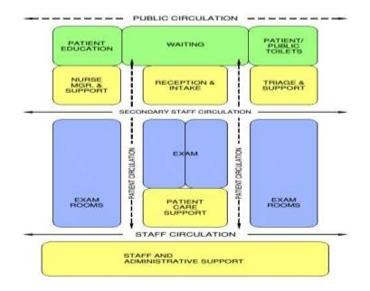
Typical Exam/Treatment Module is based on 1 0 to 1 9 exam rooms and support spaces. Rooms are arranged along double loaded corridors.
